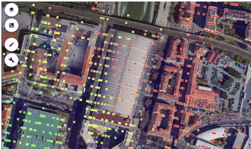
Figure 3 – Verifying Street-Level Subsidence in Gattières, France
